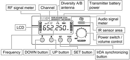
First turn on the power and the LCD display will show last stored channel and frequency. Select a channel that corresponds to the transmitter. When transmitter is turned on, the A/B diversity antenna will appear to denote that it is connected.
