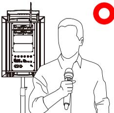
■ Locate the wireless amplifier between the speaker and the audience with the speaker facing the crowd. Place the wireless amplifier on a tripod stand and above the head of audience (about 180cm).
